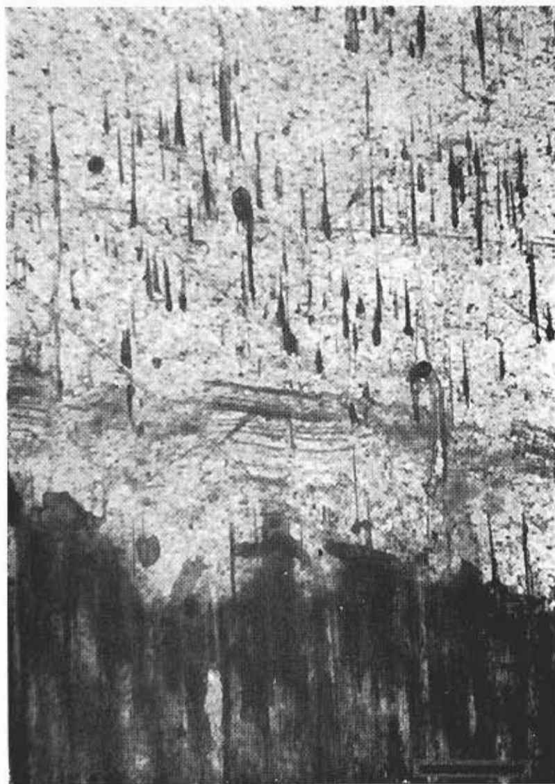
Fig. 5 - Different types of growth layers in close association. There are large, thorn-shaped inclusion defined layers, pseudo-pleochroic layers with a laminated-like banded appearance and concentration of abundant impurities that dominate the lower portion of the figure. Plane polarized light. Scale is 0.5 mm.
