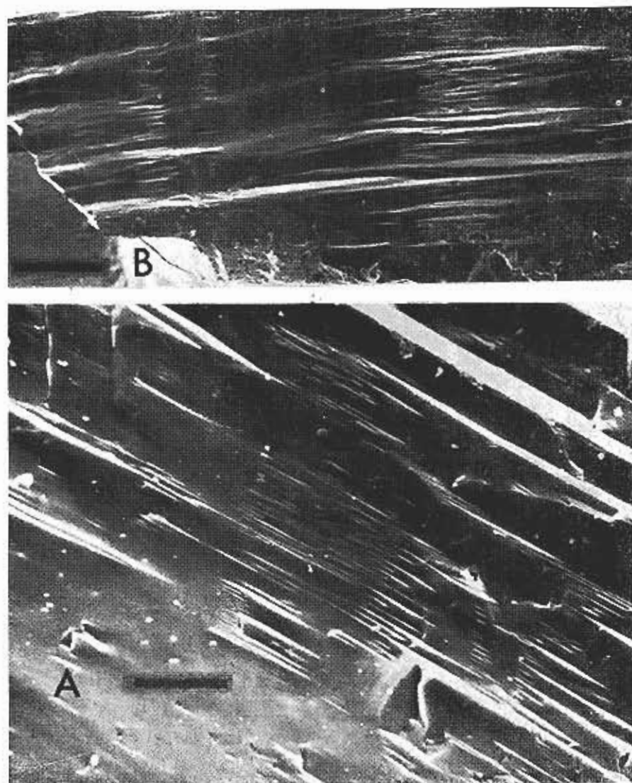
Fig. 10 - Two fracture surfaces of columnar calcite crystals showing inclusion traces that appear as spindle-shaped depressions and linear striations. These are interpreted as the remnant spaces between partially coalesced crystallites, and their mergence into larger crystals. Note the regularity and spacing that define a growth layer. Scanning electron micrographs. Scales are 20 microns (A) and 500 microns (B).
